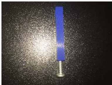
Tensioner pin printed at 155% scale, with loose screw placed inside opening.
